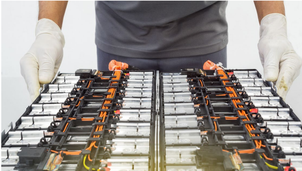
Figure 9. Used lithium-ion battery undergoing repair.
