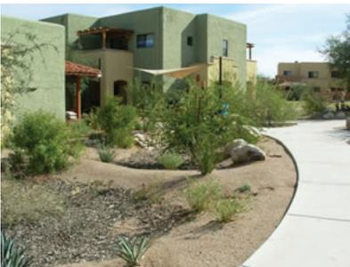
In addition to landscape use, as in this passive approach where rainwater is directed to the landscape, properly filtered and treated harvested rainwater can be used for other uses, such as toilet flushing.
